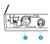
The audio outputs are available as a balanced XLR-3M output ? and an unbalanced BNC output 3, allowing you to simultaneously connect two devices (amplifier, etc.). Both outputs deliver the same output voltage, are short-circuit proof and decoupled from each other.
